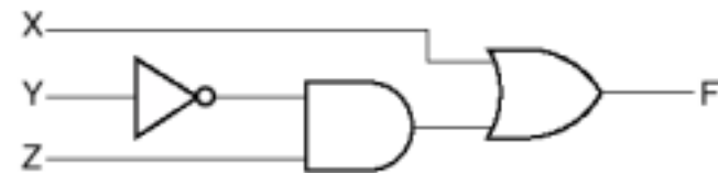
Fig. 2-3 Logic Circuit Diagram for F = X + \bar{Y}Z
