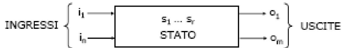
$$o_i = f_i(i_1, \dots, i_n, s_1, \dots, s_r) \quad i=1, \dots, m$$
